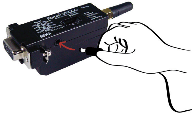
Figure 2-2 Connecting Power to Parani-SD1000
