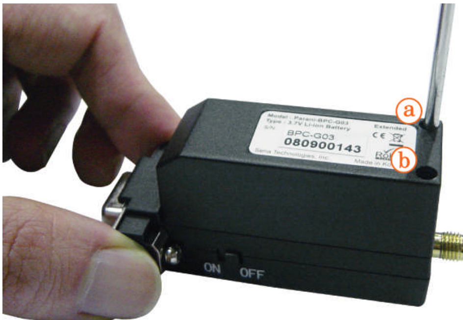
Figure 2-7 Fasten the battery pack
