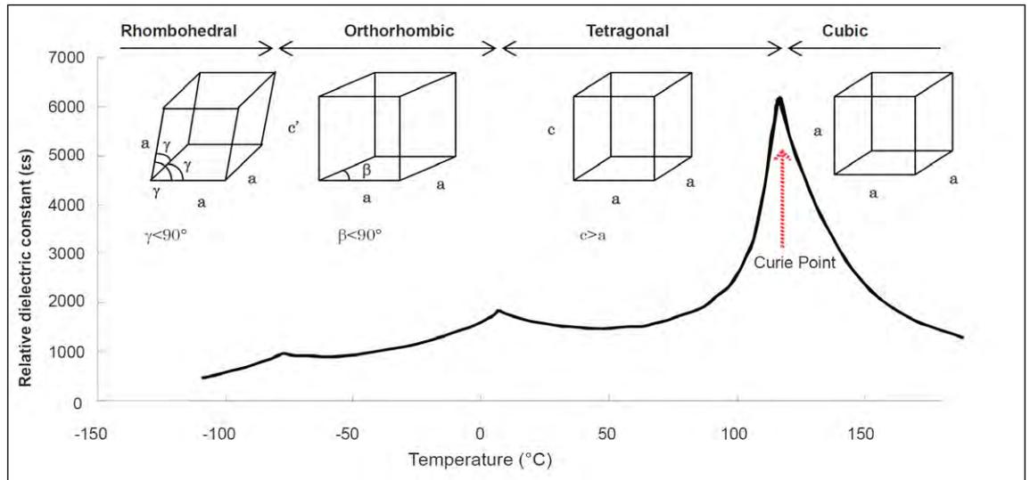
Fig. 2: Change in crystalline structure and relative dielectric constant on temperature change (pure BaTiO<sub>3</sub>)
