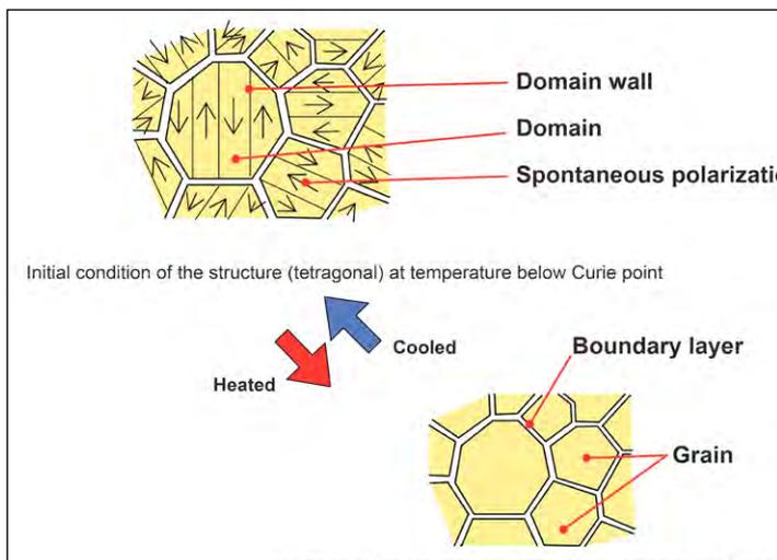
Fig. 3: Micro structure of BaTiO<sub>3</sub> type ceramics
