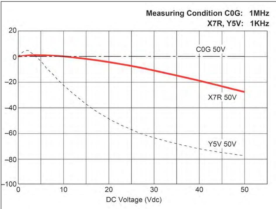
Fig. 4: Capacitance - DC Voltage Characteristics
