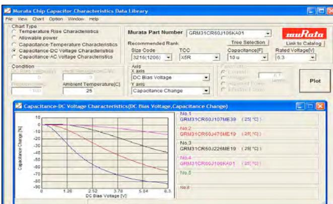
Fig. 5: Example of varying capacitance value and example of varying case size with voltage rating
