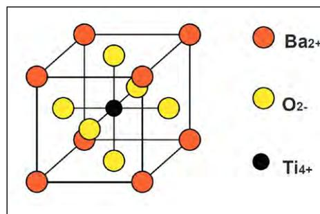
Fig. 1: Crystalline structure of  $\text{BaTiO}_3$  ceramics
