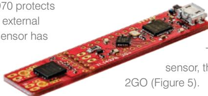
An easy-to-use design kit is available for the TLI4970 current sensor, the Current Sensor 2GO (Figure 5).
