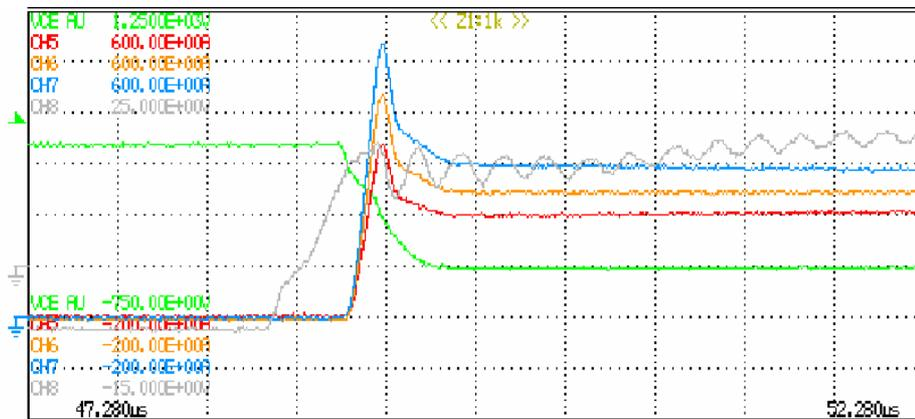
Fig. 8: Three half-bridges EconoPACK<sup>TM</sup>+ in parallel. Current sharing without matching. [Courtesy General Electric Co., Salem VA]
