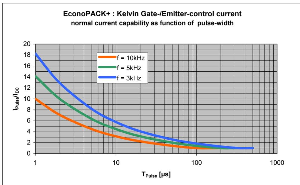
Fig. 12: Auxiliary collector, gate and auxiliary emitter load table EconoPACK<sup>TM</sup>+
