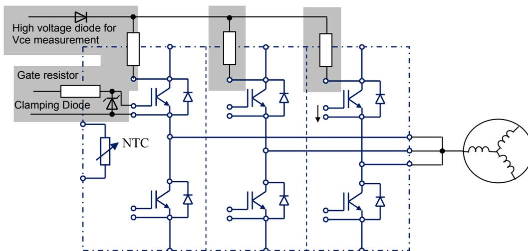
Fig. 11: Drive circuit EconoPACK™+ in parallel.
