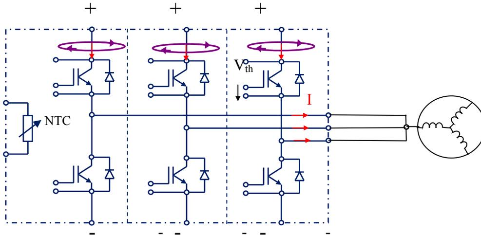
Fig. 6: Magnetic fields with paralleled EconoPACK™+
