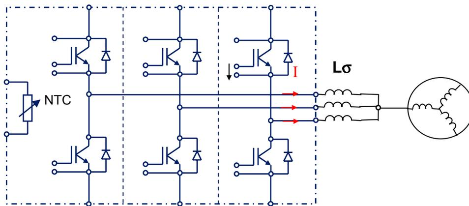
Fig. 14: Symmetry by means of output inductors.
