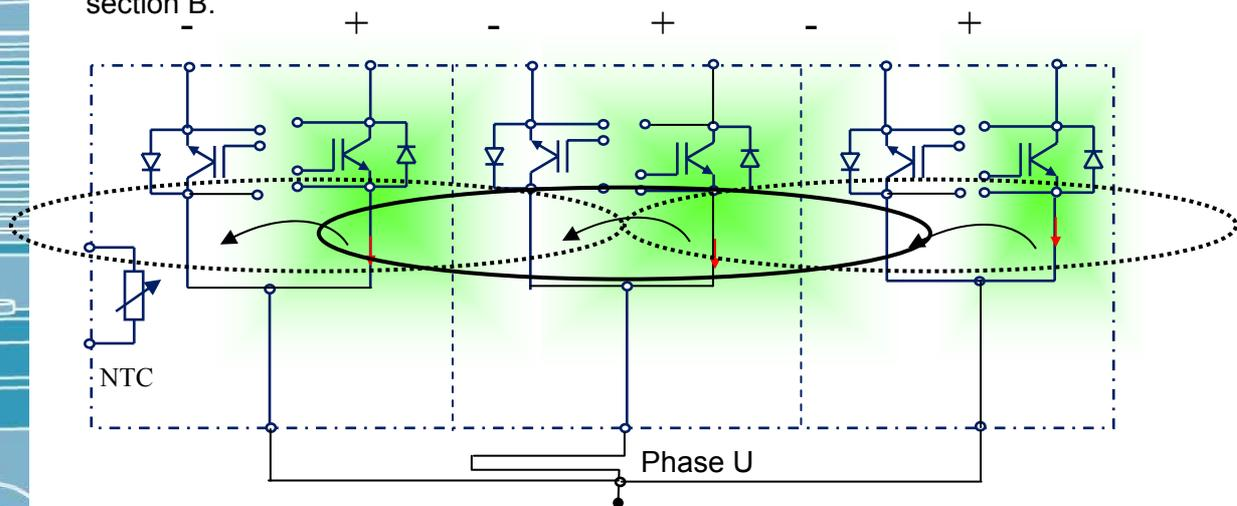
Fig. 7: Commutation process for paralleled EconoPACK™+ .
