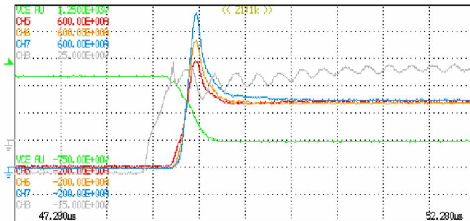
Fig. 9: Three half-bridges EconoPACK<sup>TM</sup>+ in parallel. Current sharing during turn on by matching gate resistors. [Courtesy General Electric Co., Salem VA]
