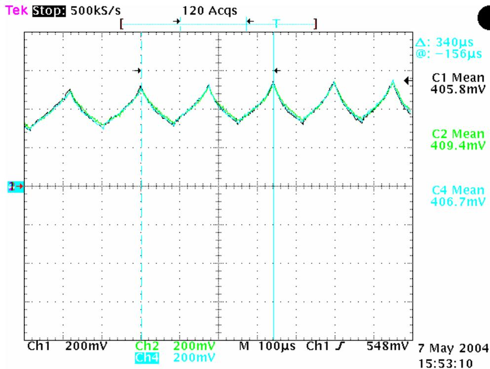
Fig.19: Current sharing in the triple parallel circuit with EconoPACK<sup>TM+</sup>. Measured at the three output phases  $\Sigma 1410A$ .
