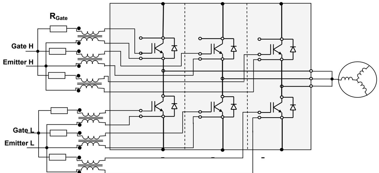
Fig 13b: Current limitation in the aux. leads by current compensating chokes.
