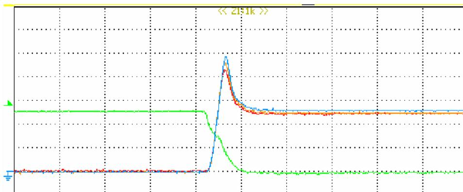
Fig. 10: Three half-bridges EconoPACK<sup>TM</sup>+ in parallel. Current sharing by matching the DC-bus stray inductance. [Courtesy General Electric Co., Salem VA]
