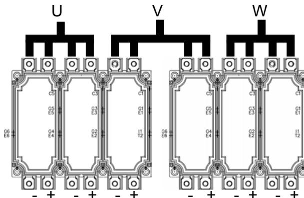
Fig. 2 : Dual parallel connection
