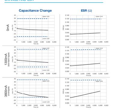
Hybrid capacitors exhibit high reliability when subjected to high ripple currents. In recent testing, the capacitors had the electrical characteristics at no load and rated ripple current (1,300mA) conditions. At three times the rated ripple current (3,600mA), the capacitor's electrical characteristics did change, but no shortage took place.
