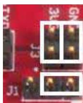
**Figure 6. USB (eZ-FET) Power Jumper Configuration**
