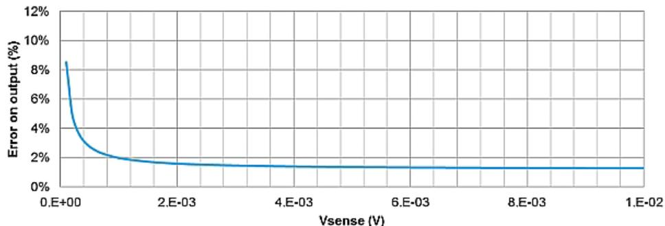
*Figure 3: Total error assuming 0.1% resistances with Rshunt 1%*
