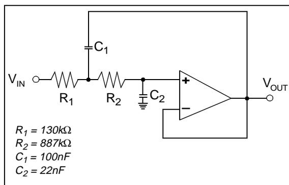
**FIGURE 6:** This Sallen-Key, 2nd order, 10Hz, Butterworth, low pass filter circuit has two large resistors in series with the non-inverting input of the op amp. Input bias current errors from a Bipolar op amp will cause a considerable amount of error. In contrast, the input bias current from CMOS or BiFET amplifiers will be low enough not to cause appreciable errors.
