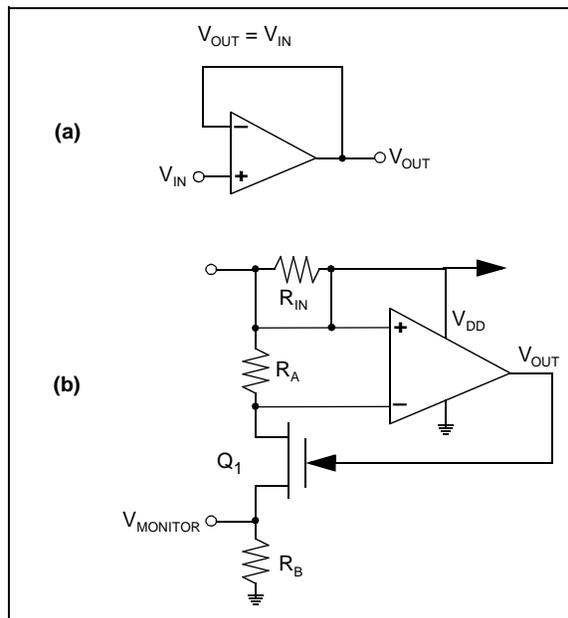
**FIGURE 8:** If an amplifier is used as a buffer (a), the input devices of the operation amplifier may limit the input range of the buffer. If an amplifier is used in a high power supply sense circuit (b), the input stage must be able to extend to the positive rail.
