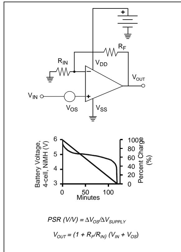
**FIGURE 9:** A battery powered application can see a change in power supply voltage of several hundreds of millivolts over the life of the product. If an op amp is configured with a high closed loop gain in these types of applications, it must have good DC power supply rejection.
