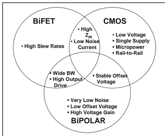
**FIGURE 2:** Different IC processes render different advantages for amplifiers. The choices in processes for single supply amplifiers are Bipolar, CMOS and BiFET, which is a combination of Field Effect Transistors (FET) and Bipolar transistors.
