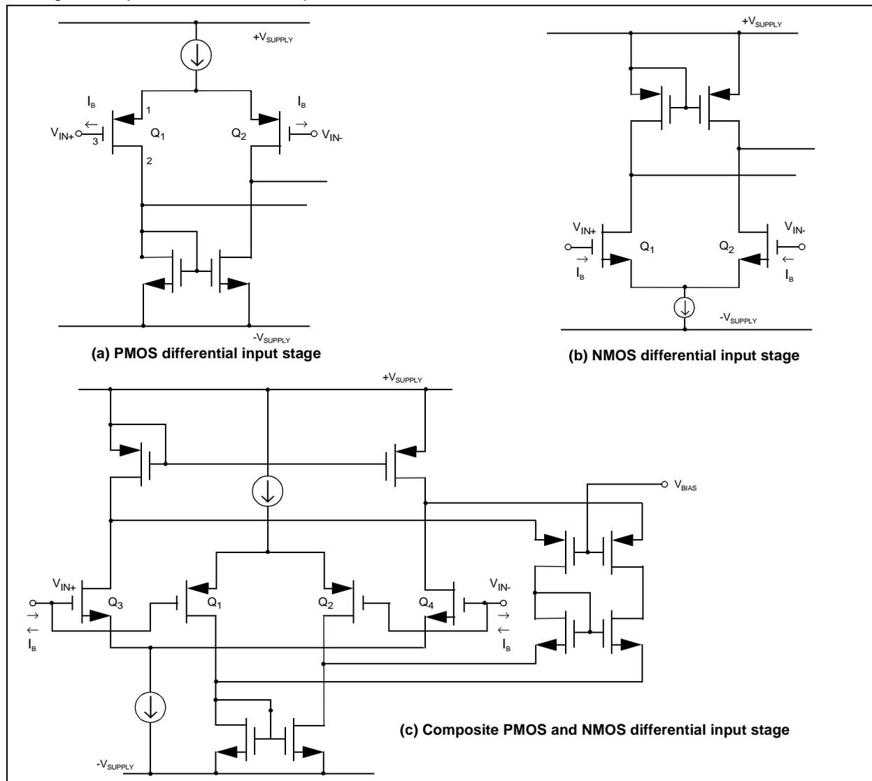
**FIGURE 7:** The input voltage range of an op amp is dependant on the topology of the input stage of the amplifier. The input stage can be constructed of PMOS (a) devices allowing for the input to swing below the negative supply or a NMOS differential pair (b) where the inputs can swing above the positive supply. A composite input stage (c) uses PMOS and NMOS differential pairs so the input voltage range can extend from above the positive rail to below the negative rail.
