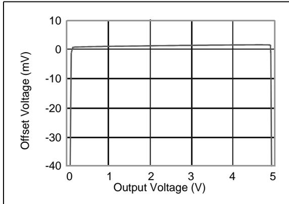
**FIGURE 11:** This graph shows the relationship between the output swing of an amplifier and input offset voltage with a  $25k\Omega$  load and  $V_{DD} = 5V$ . The open loop gain of the amplifier can be calculated by selecting two points on the graph and calculating the slope. As the output swing of the amplifier goes towards the rail, the amplifier function eventually breaks down. This is first manifested with changes in input offset voltage.
