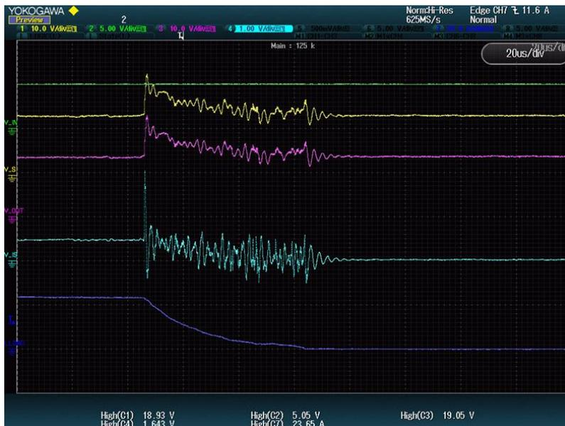
**Figure 6 Loss of Load – BTS50010-1TAD scope plot example**
