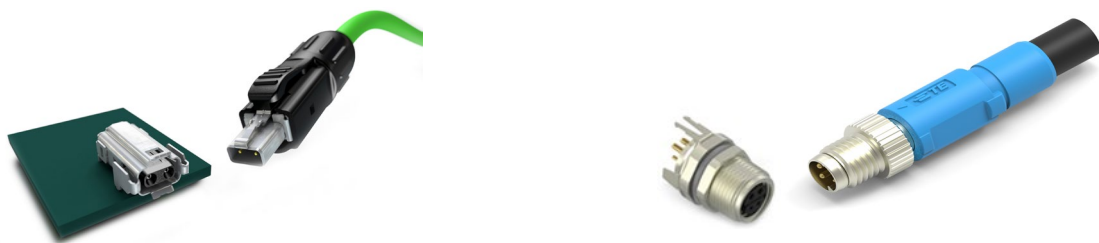
Figure 1: Single Pair Ethernet connectors per IEC 63171-6: (a) IP20 connector for SPE where power may be delivered via PoDL with max. 1,36 A (b) IP67 hybrid connector for SPE with separate power contacts allowing for currents up to 8 A
