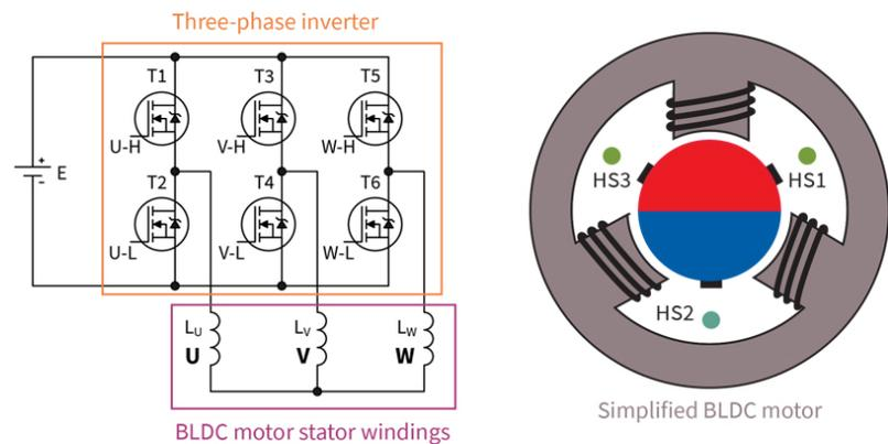
Figure 1: Three-phase BLDC motor drive overview
