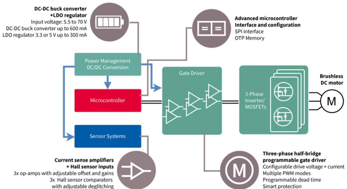
Figure 3: Overview of the 6EDL7141 smart three-phase motor gate driver
