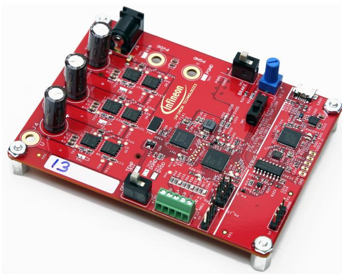
Figure 5: Infineon's advanced motor drive evaluation board
