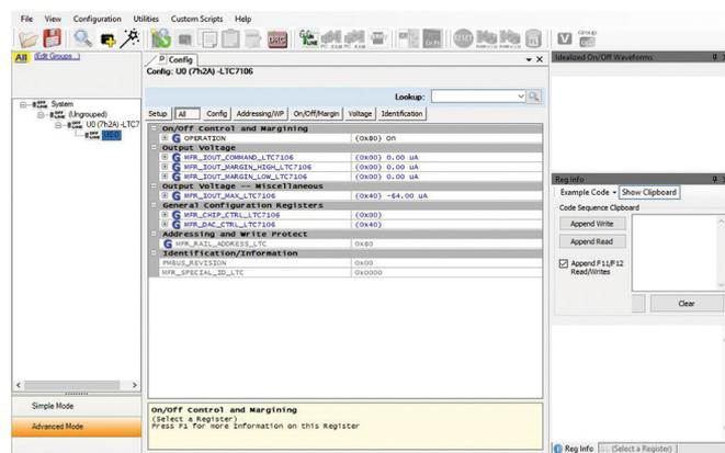
Figure 3. The LTPowerPlay graphical user interface for controlling the LTC7106 via a PMBUS or I<sup>2</sup>C.
