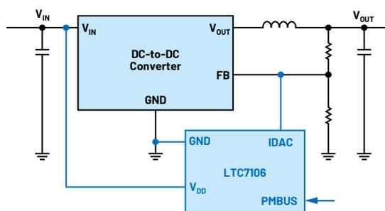
Figure 2. An LTC7106 DAC for dynamically adjusting the output voltage of a switching regulator.
