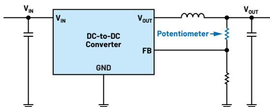
Figure 1. Switching regulator with potentiometer in the resistor path for adjusting the output voltage.
