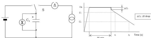
$C = \frac{I \times (t_2 - t_1)}{U_1 - U_2}$ |
