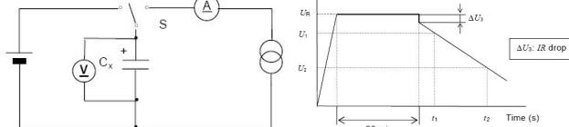
$C = \frac{I \times (t_2 - t_1)}{U_1 - U_2}$ |
